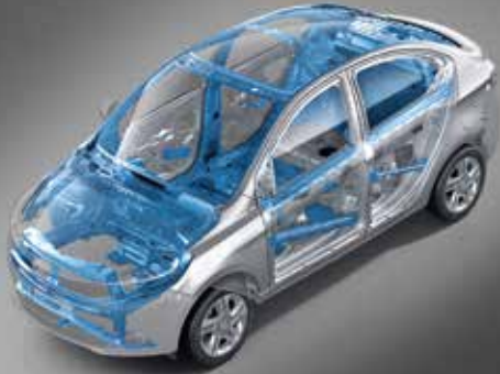
ENERGY ABSORBING STRUCTURE
